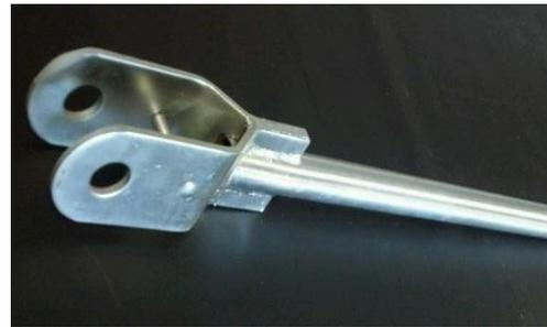
4. Slide both upper arms into the aluminum / steel pivot arms (make sure that both arms end up the same length) and lightly tighten the two bolts that hold each upper arm in the pivots. Final tightening will be done later.
